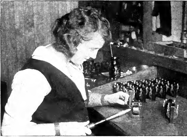
SOLDERING TRANSFORMER LEADS—A DELICATE JOB
